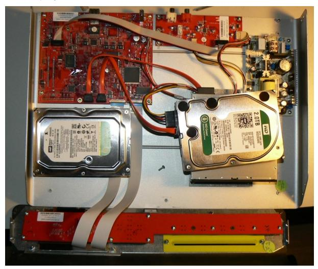
After success of the recovery, I removed the original harddisk with the bolts on the bottom (size 2 mm bit). The rubber feets can be removed from the harddisk by turning them counter clockwise (like a normal bolt). Now everything in reverse for installing the harddrive.
