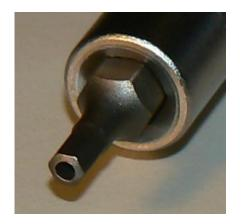
For the cover screws size 1/8 inch is required. For the removal of the harddisk size 2 mm is needed.
