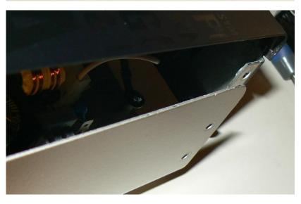
On the back, a connector to the power supply and the ground connection via a bolt to the chassis needs to be removed.
