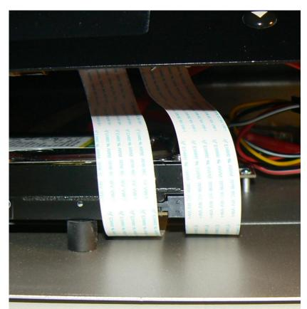
On the front, 2 delicate ribbons are connecting the LCD screen and buttons to the main board. I did not see any connector types and I did not want to mess with it either. It looks more delicate than the connection in the Opus 4.
